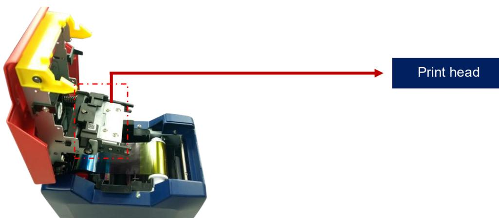
Step 3: Wipe the print head in one direction, from left to right or right to left with cleaning stick. Do not wipe back and forth. Generally wipe 3-5 times will be ok.
