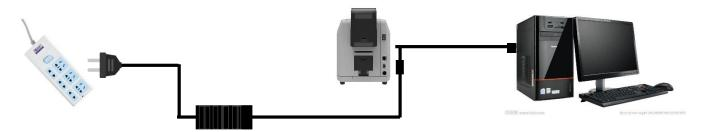
Power adapter 24V connector is inserted into card printer power interface. Connect the power cable to the power adapter. Then plug the power cable into the mains socket. But do not power on until the driver installation is complete.
